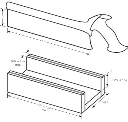
*Note:* The boards must not be less than <sup>5</sup>/8" thick.
