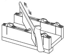
Caution: The saw must be inserted between the guides rather than from the top; otherwise, the set in the teeth will be damaged.
