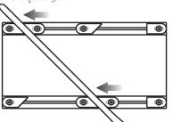
Caution: The saw must be slid out of the guides rather than lifted out; otherwise, the set in the teeth will be damaged.
